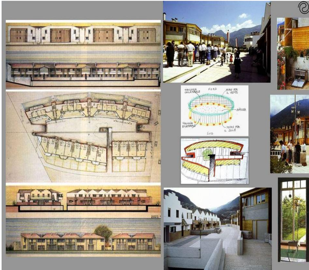
Figure 18. To understand how thinking by image can produce interesting inferences, we can observe the schematic drawing at the center where we recognize the double asymmetry of the square and the building; the first inverted compared to the second. In the buildings, a façade opens into the sun with a portico on the south side, and a façade with a wall protects from wind on the north side. Vice versa, the square, as a room without ceiling, has a north façade open to the sun and a south one that is protected. Thus, the façades do not merely perform but rather make communicable the sense of opening and protection using “architectural words”. This case gives us the opportunity to show how exemplificative inference works. In fact, it fulfills the double task of instantiating a built form while, at the same time, highlighting some of its properties. The iterated use of such a selection, related to the life form of a symbolic community, makes it permanent. Therefore—as it happens in language—it is a selection made by the community, not by an individual. This happens with color and cloth in the samples as conventional association of the cloth sample (the swatch) with the cloth of a dress.
