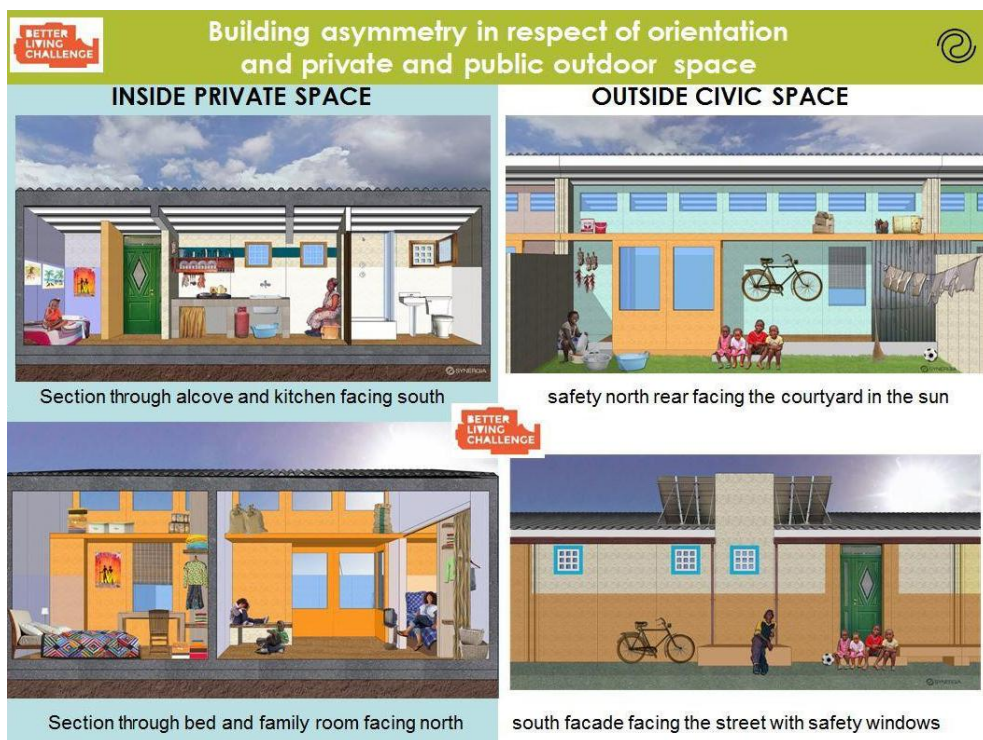
Figure 12. This house is small, flexible, and self-constructed by recycling energy-efficient material. The images show the double asymmetry of these buildings: one asymmetry is about the orientation toward north and south exposure and the other is about community, i.e. public outdoor space and private interior space (Image by Synergia Studio, 2014).
