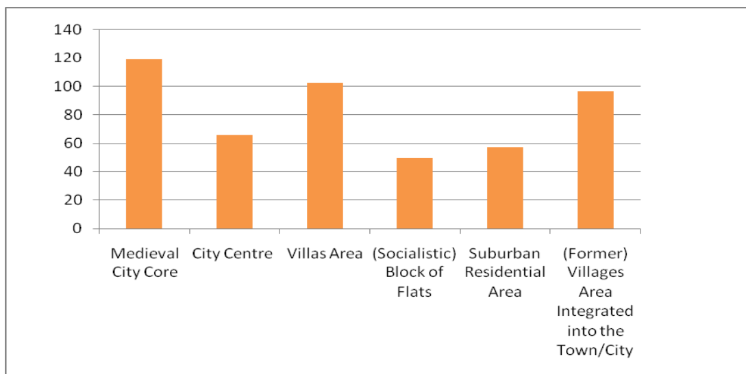
Graph 3 Comparison of the Costs of Construction Recalculated per 1 Resident according to Individual Types of Spatial Structures (adapted from Malířová 2012).
