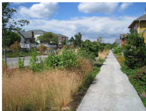
Image 11. Bio-swales provide a way to protect, even improve, ecological function in urban watershed systems. Seattle, Washington.
